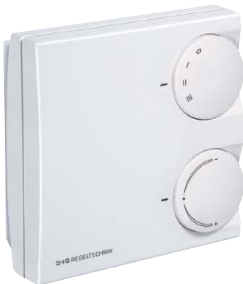
RTF xx PD (Balduur 2) Version with sensor, potentiometer (1 kOhm, max. 0.1 W) and and turn switch (max. 24 V AC/DC, max. 130 mA)
