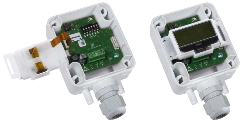
PREMASGARD® 112x Pressure connectors on the bottom side, with display
