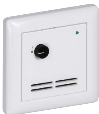
FSTFxxLD2 Version with sensor, LED (green), and turn switch (2-step) (max. 24 V AC/DC, max. 130 mA)
