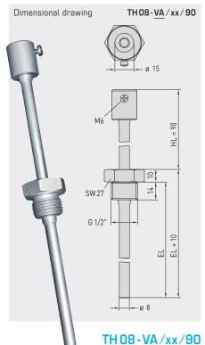
Immersion sleeve, stainless steel V4A (1.4571) with neck tube
