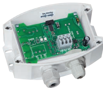
PLGF-U with output 0-10V, UB = 24V
